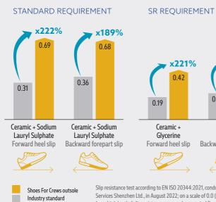
Slip resistance test according to EN ISO 20344:2021, conducted by Intertek Testing Services Shenzhen Ltd., in August 2022; on a scale of 0.0 (without slip resistance) to 1.0 (very high level of slip resistance, e.g. on dry carpeted floors). All SFC shoes are fitted with the patented, slip-resistant Shoes For Crews outsole
